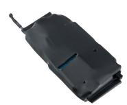
**STronic URP GSM K+** is a device which is a combination of 2 different modules, Listening module GSM based and then Voice Recording module with VOX activation only. To access the devices recordings, you have to connect it to a PC and physically get the data.
